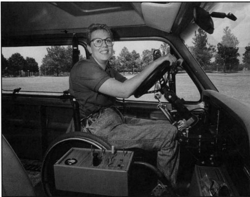
Sue Johnson-Smith demonstrates a zero-resistance steering mechanism and a console on which extended handles allow her to control lights, turn signals, windows, and other electrically-controlled features of the van.
