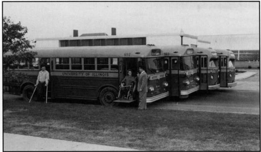
The 1956 GMCs and Marmon-Herrington buses were the first to have wheelchair lifts and steps at the front door so that ambulatory and wheelchair individuals can enter and leave quickly and safely.
